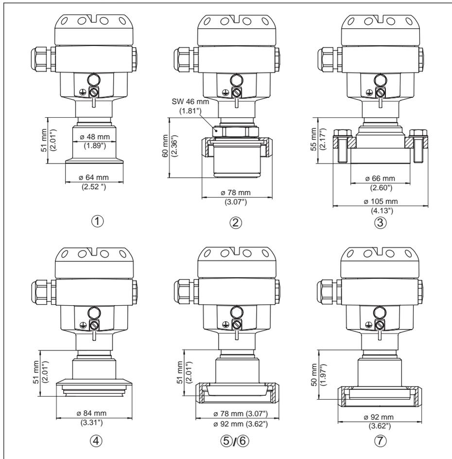
Fig. 53: CPT-2x, raccord aseptique
