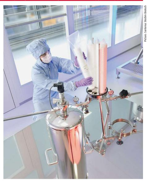
One of the applications for pressure sensors with in-line diaphragms: measuring pressure drop across cartridge filters.
