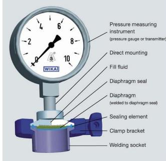
A diaphragm seal between the pressure gauge or sensor eliminates dead space and allows the vessel or pipe to be sterilized without damaging the measuring element.
