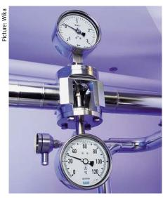
In sanitary applications it is important to make sure that the fill fluid behind the diaphragm is compatible with the process fluid, in case the diaphragm is damaged.
